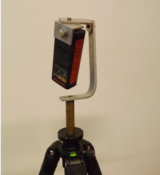
Fig. 8. Tripod-head for DistoX2
